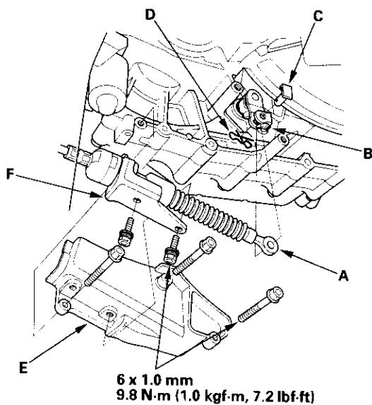
25. Install the shift cable cover (E), then secure the shift cable holder (F) to the shift cable cover with the bolts.
