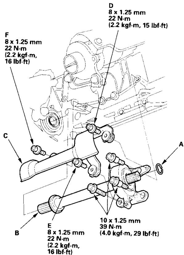
13. Clean the areas where the intermediate shaft contacts the transmission (differential) with solvent or carburetor cleaner, and dry with compressed air. Then install the intermediate shaft in the differential. While installing the intermediate shaft, be sure not to allow dust or other foreign particles to enter the transmission.
