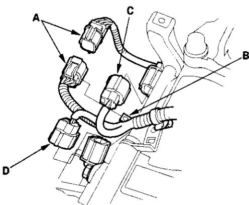
41. Connect the connectors to the mainshaft speed sensor (C) and countershaft speed sensor (D).
