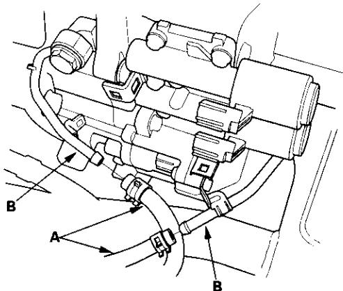
38. Connect the shift solenoid harness connector (A), A/T clutch pressure control solenoid valve B connector, and solenoid valve C connector. Install the harness clamps (D) on the clamp brackets. (E).
