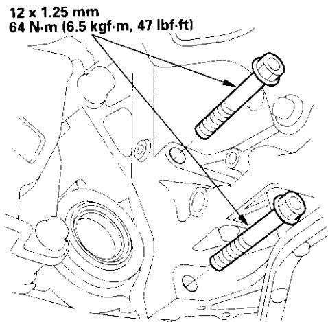
9. Install the transmission housing mounting bolts.
