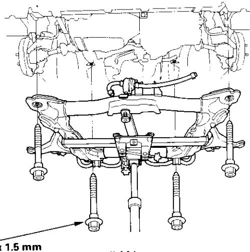
20. Align the reference marks (A) with the center of the subframe mounting bolt heads (B), then tighten the bolts to the specified torque.
