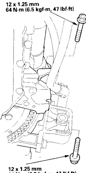
10. Install the transmission housing mounting bolts.
