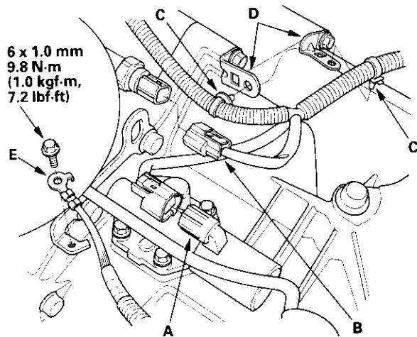
43. Install the transmission ground terminal (E).
