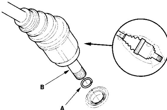
17. Install the right and left driveshaft (see page 16-16). While installing the left driveshaft in the differential, be sure not to allow dust or other foreign particles to enter the transmission.
