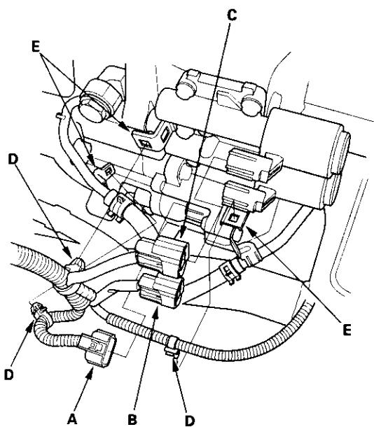
39. Connect the 3rd clutch transmission fluid pressure switch connector.
