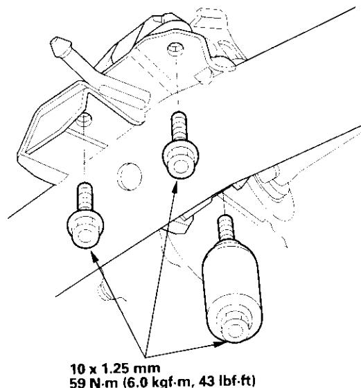
22. Install the front mount bolt (A) and nut (B), connect the ATF cooler hose (C) to the ATF cooler pipe.
