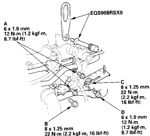
34. Install the brake booster and EVAP line bracket mounting bolts (A) and air cleaner housing bracket mounting bolt (B).
