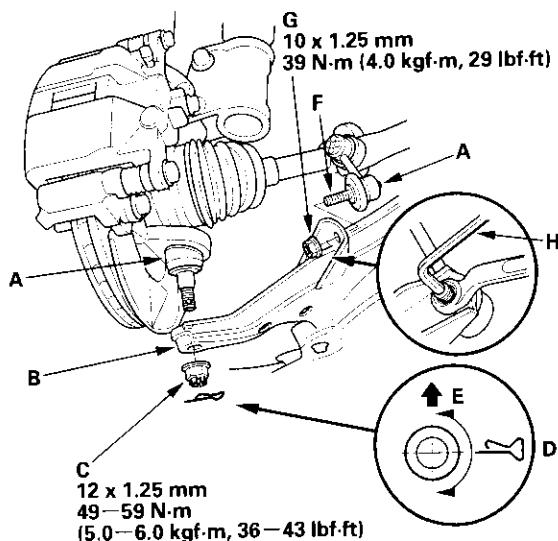
31. Connect the ball joints (F) to the lower arms, and install the nuts (G). Insert a 5 mm Allen wrench (H) in the top of the ball joint pins, and tighten the nuts.
