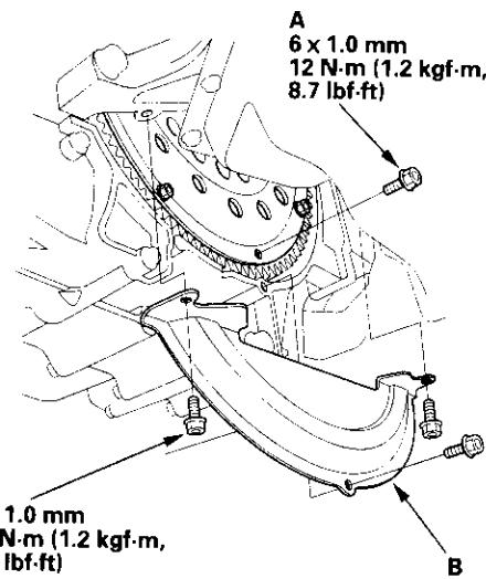
27. Install the torque converter cover (B).
