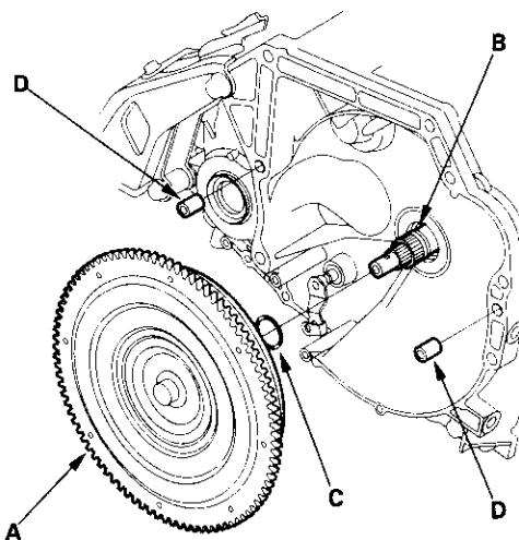
6. Install the 14 x 20 mm dowel pins (D) in the torque converter housing.
