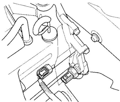
40. Connect the transmission range switch connector (A), and install it on its bracket (B).
